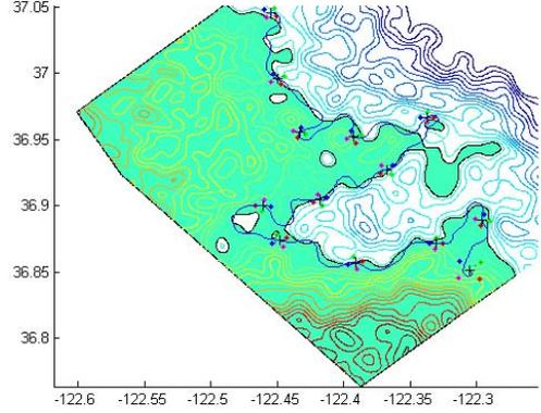
Fig. 3. Tracking the temperature level curve of 14.25°C in an estimated temperature field near Monterey Bay, CA on August 13, 2003. For visualization purpose, the level curve is accentuated. The trajectory of the center of formation is plotted with status of the formation shown along the trajectory. The horizontal axis corresponds to longitude and the vertical axis to latitude.
