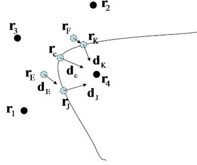
Fig. 1. Detection of a level curve using four sensor platforms.  $\mathbf{r}_c$  denotes the center of the entire formation.  $\mathbf{r}_E$  denotes the center of the formation formed by  $\mathbf{r}_1$ ,  $\mathbf{r}_3$  and  $\mathbf{r}_4$ .  $\mathbf{r}_F$  denotes the center of the formation formed by  $\mathbf{r}_2$ ,  $\mathbf{r}_3$  and  $\mathbf{r}_4$ .  $\mathbf{r}_j$  and  $\mathbf{r}_k$  are located on the same level curve with  $\mathbf{r}_c$ .
